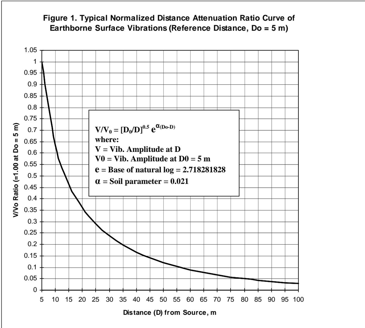
The curve is representative of many locations in the L.A. Basin, and also of various locations in Sacramento, and can be used for estimating traffic, train, and most construction vibration drop-offs with distance. To use the curve, the vibration amplitude  $V_1$  must be known at a given distance  $D_1$  near the source, preferably between 5 and 15 m (16 and 50 ft). The vibration amplitude  $V_2$  at the distance of interest  $D_2$  can then be calculated as follows:
