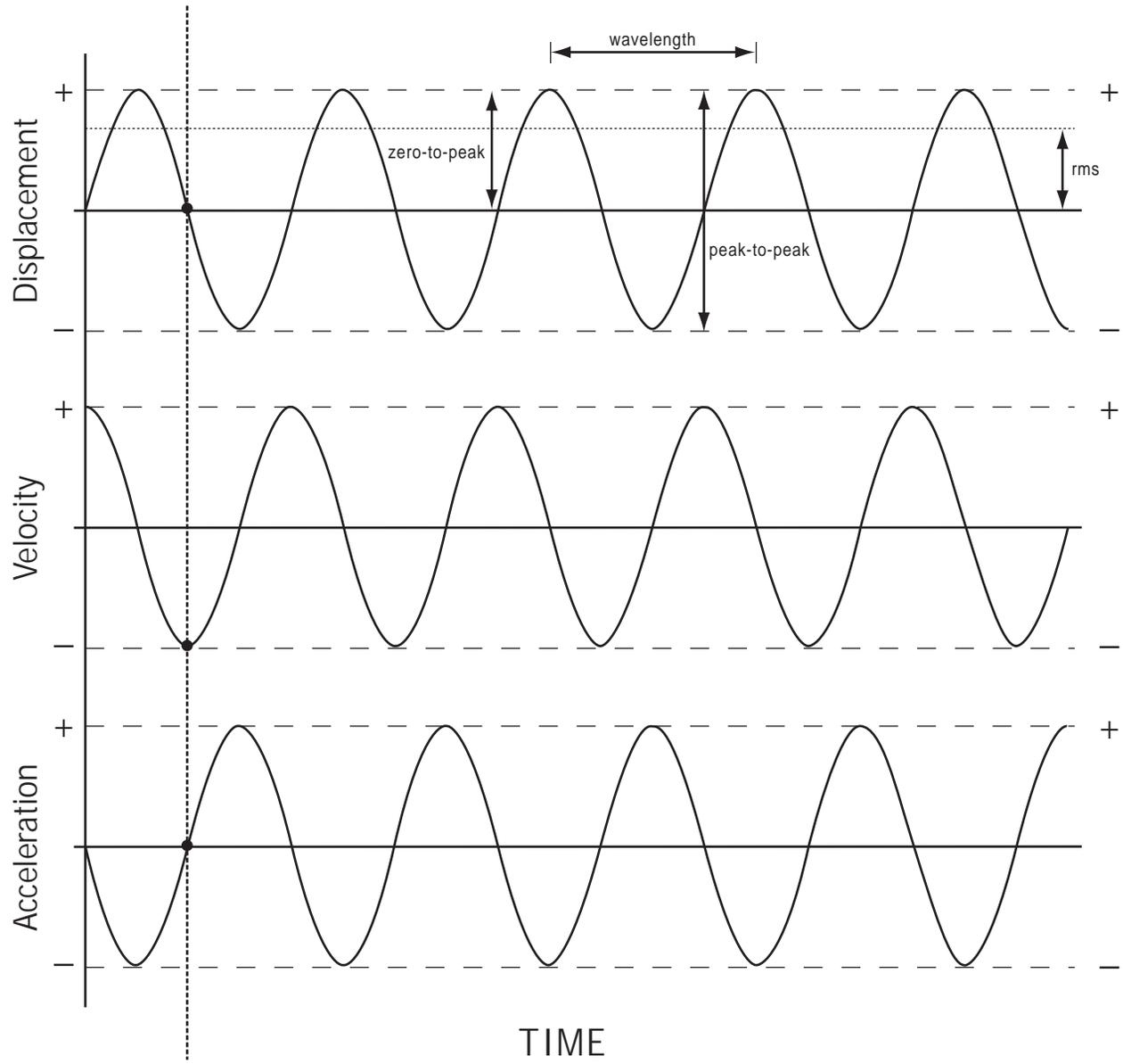
by integration (dividing by  $2\pi f$ ) and the acceleration amplitude can be determined by differentiation (multiplying by  $2\pi f$ ).
