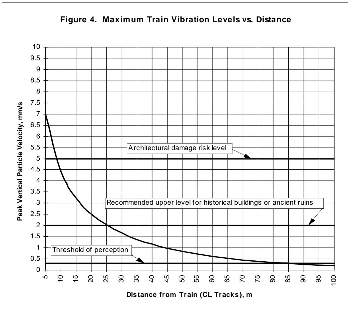
the vibration amplitude is calculated at 7 mm/s. The curve represents maximum expected amplitudes from trains, and thus is very conservative. Measurements at various distances at other locations and different freight trains averaged about two-thirds of those shown in the curve.
