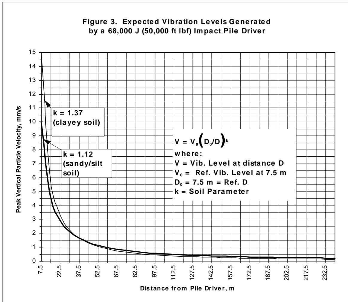
soils provide more resistance to advancing piles and therefore generate higher vibration amplitudes near the source than those in sandy soils. Vibrations in clay soils, however, tend to drop off more rapidly with distance than those in sandy soils.
