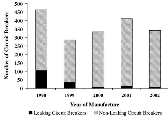
For the circuit breakers in the data set that were manufactured in 1998, 23 percent were identified as leaking. These circuit breakers account for approximately 62 percent of the total number of leaking breakers. This result is intuitive considering the natural deterioration of seals and equipment over time.
