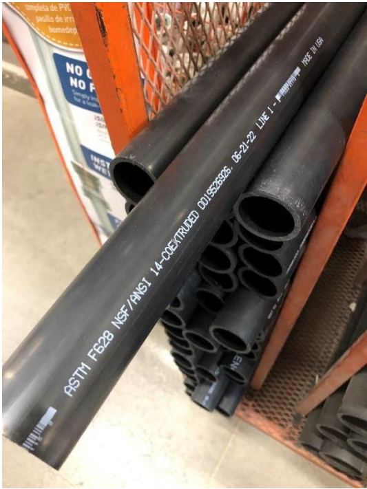
Non-potable/wastewater black PVC pipe
