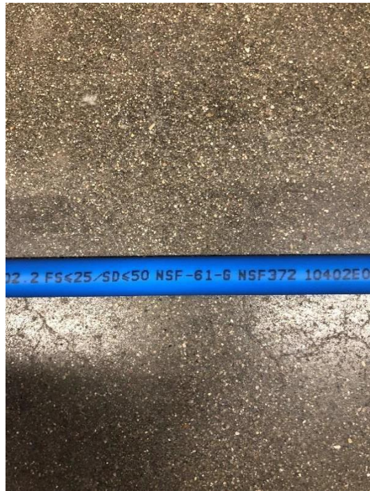
Blue potable PEX line with NSF label
