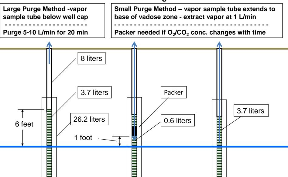
Large purge method – vapor sampled after purging well casing & sand pack Small purge method – vapor sampled after  $O_2^{t,2}/CO_2$  concentrations become stable
