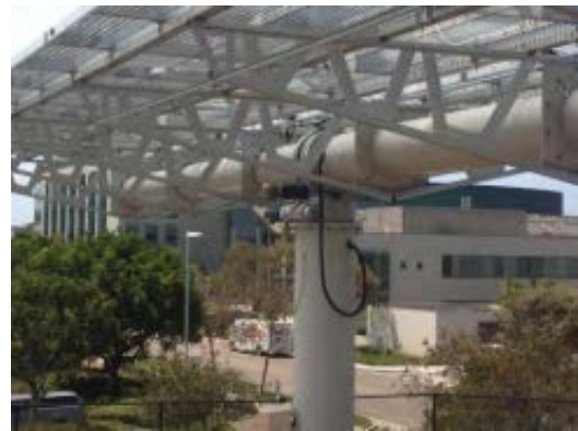
Figure 8: CPV dual-axis tracking system.
