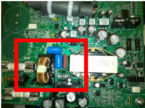
Board Level Filtering and EMI Reduction Layout
