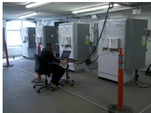
8 Hour HASS Burn-in Test and Final Verification
