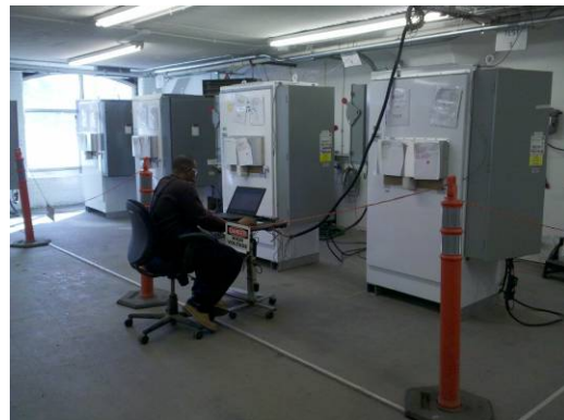
8 Hour HASS Burn-in Test and Final Verification
