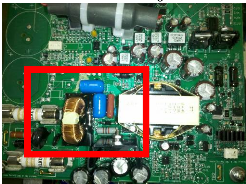
Board Level Filtering and EMI Reduction Layout
