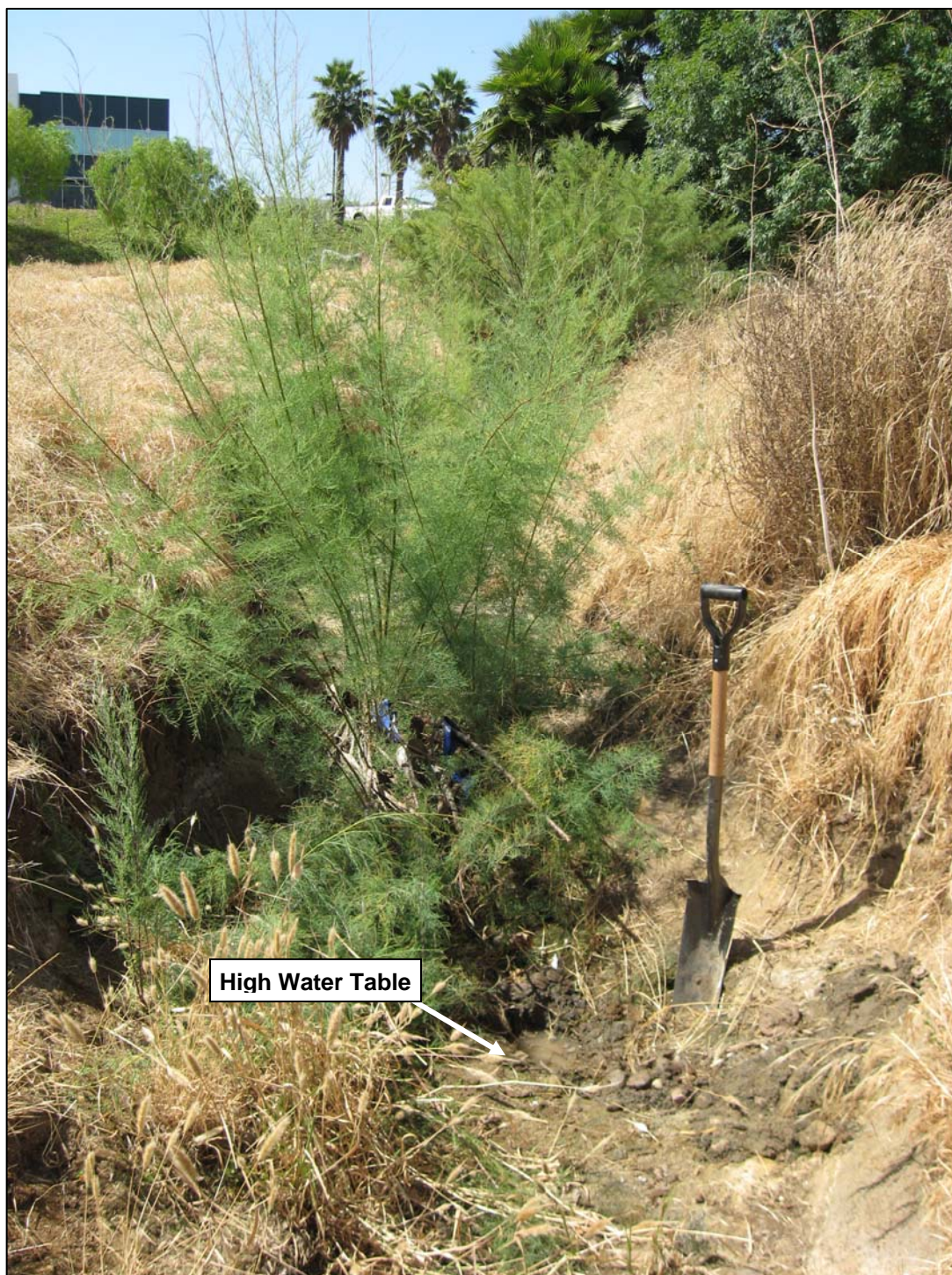
Photo A-5: Soil pit at Transect A-2 located downstream of salt cedar grove ( Tamarix sp.). High water table can be seen.
