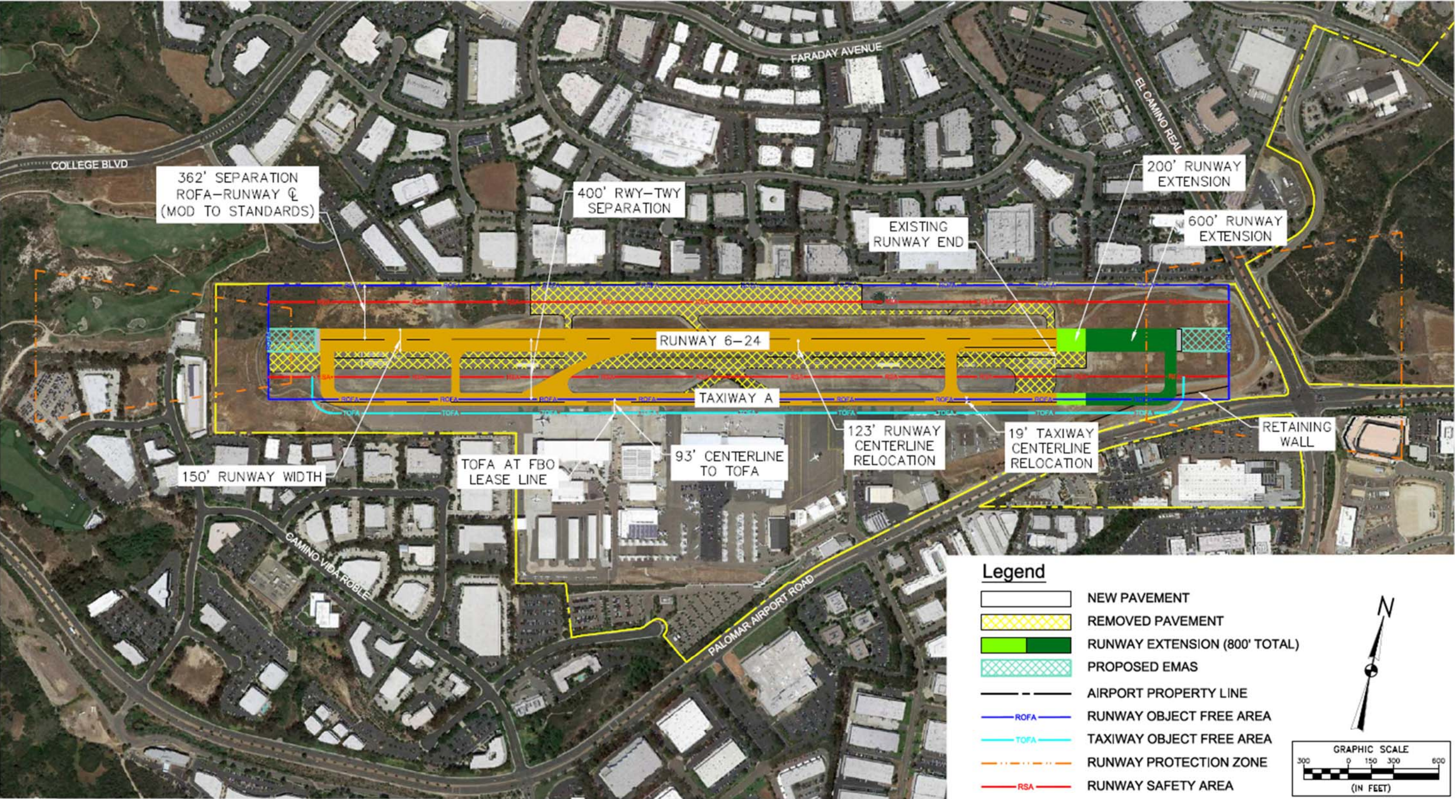
Exhibit 5.7 Airfield Alternative 6 – ARC C-III Modified Standards Compliance
