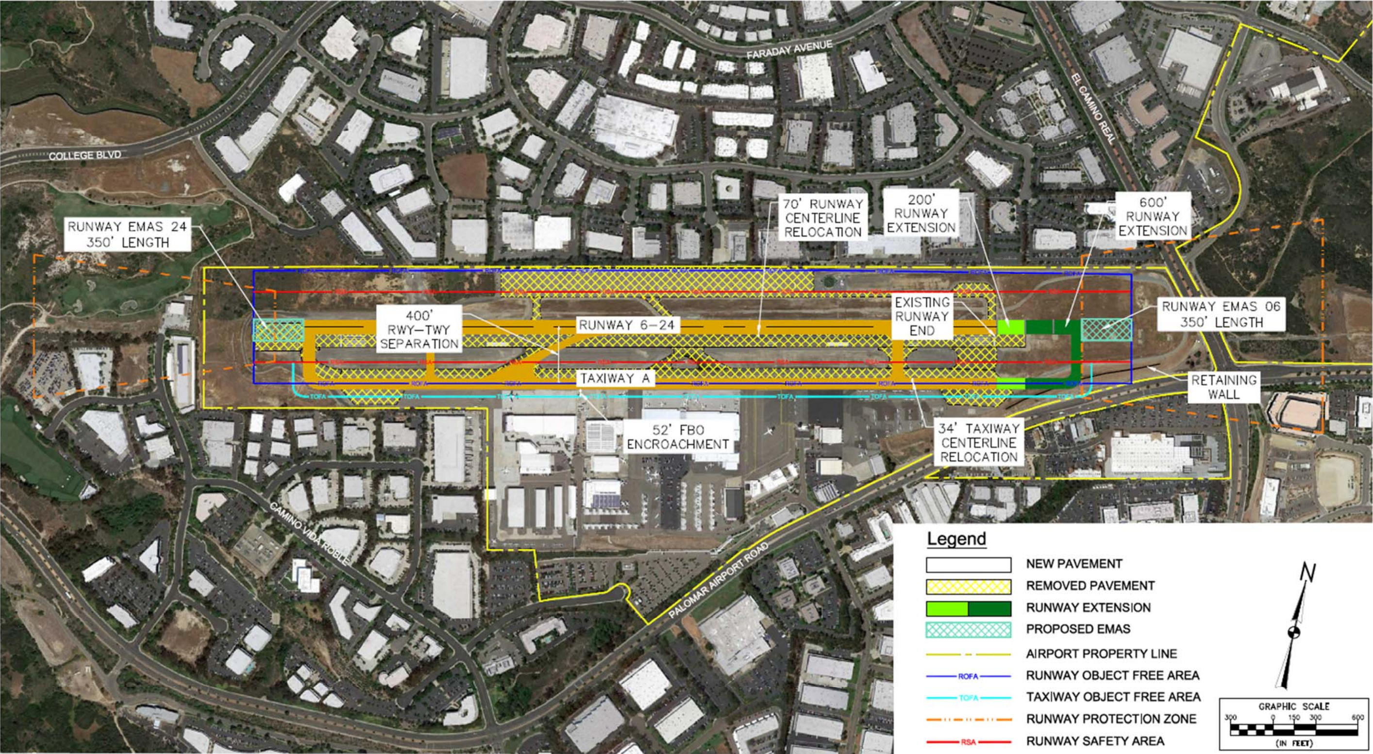
Exhibit 5.4 Airfield Alternative 3 – ARC D-III Modified Standards
