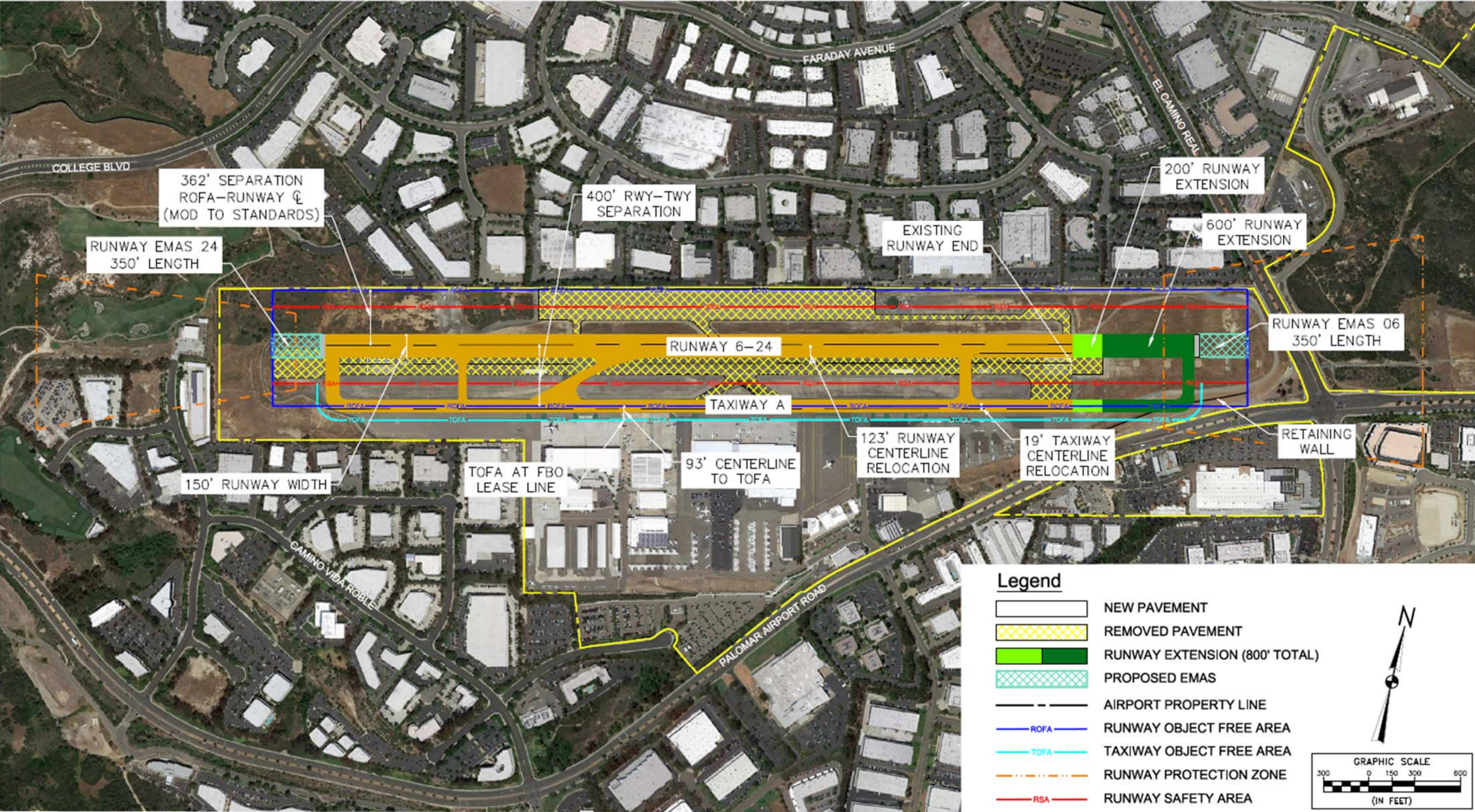
Exhibit 5.6 Airfield Alternative 5 – ARC D-III Modified Standards Compliance
