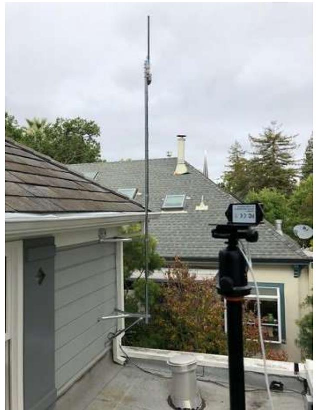
Convergence Instruments' sound-level meter installed on a rooftop in order to record airplane noise overhead. The meter automatically uploads information to the CIDataSolutions cloud data service.
