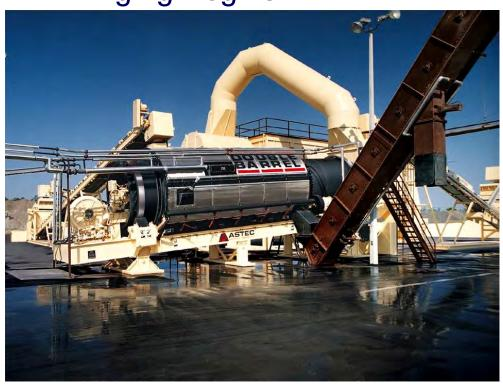
The first significant hardening of the asphalt cement takes place in the pugmill or drum mixer where heated aggregate is mixed with hot asphalt cement. During this short mixing time, the asphalt cement, which is in very thin films, is exposed to high temperatures ranging from 275 to 350° F.
