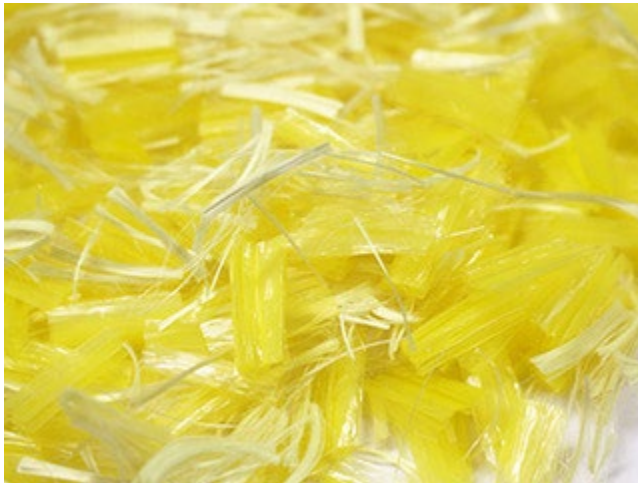
Figure 1 - Close up of Reinforced Fibers: Polypropylene and Aramid
