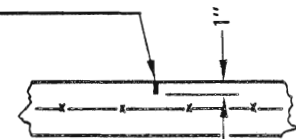
WEAKENED PLANE JOINT
