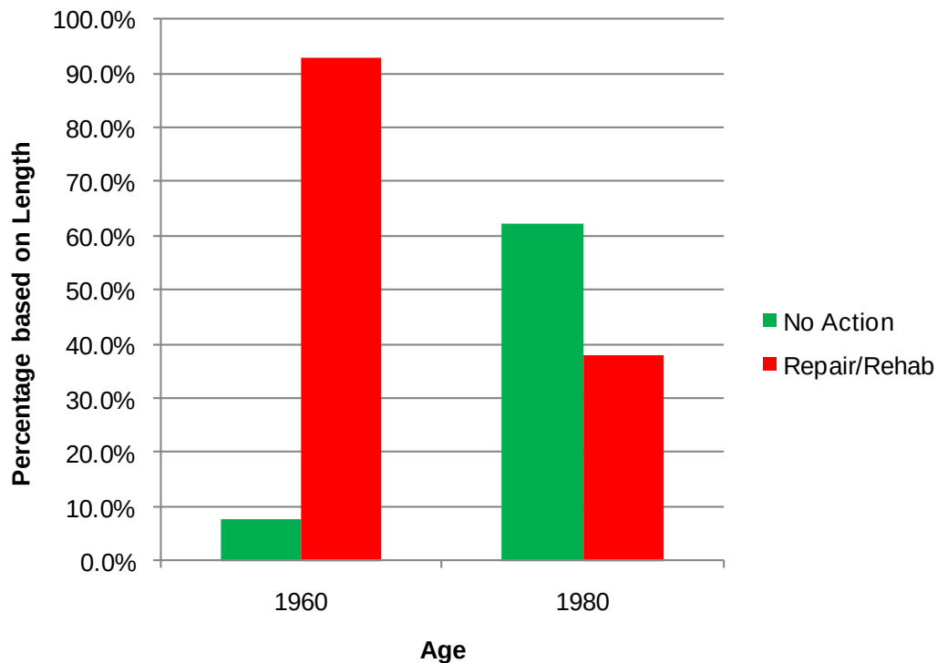
Figure 5-4 Pipeline Inspection and Assessment Findings by Age
