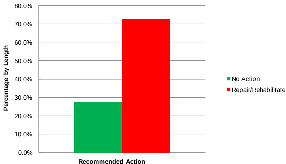
Figure 5-4 Pipeline Inspection and Assessment Findings by Percentage of Length
