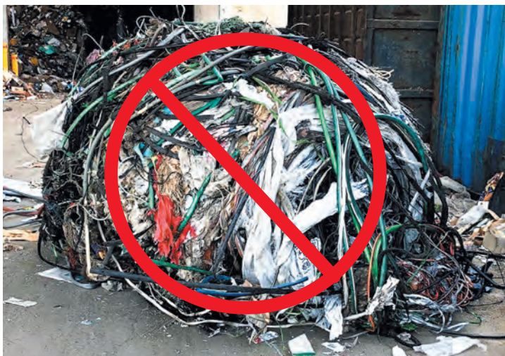
These "tangles" were pulled out of sorting machinery at a Material Recovery Facility.
