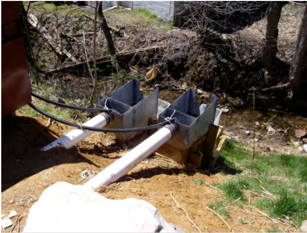
Figure 4-15. Underdrains from permeable pavement equipped with 30° V-notch weir boxes and samplers for flow and water quality monitoring.
