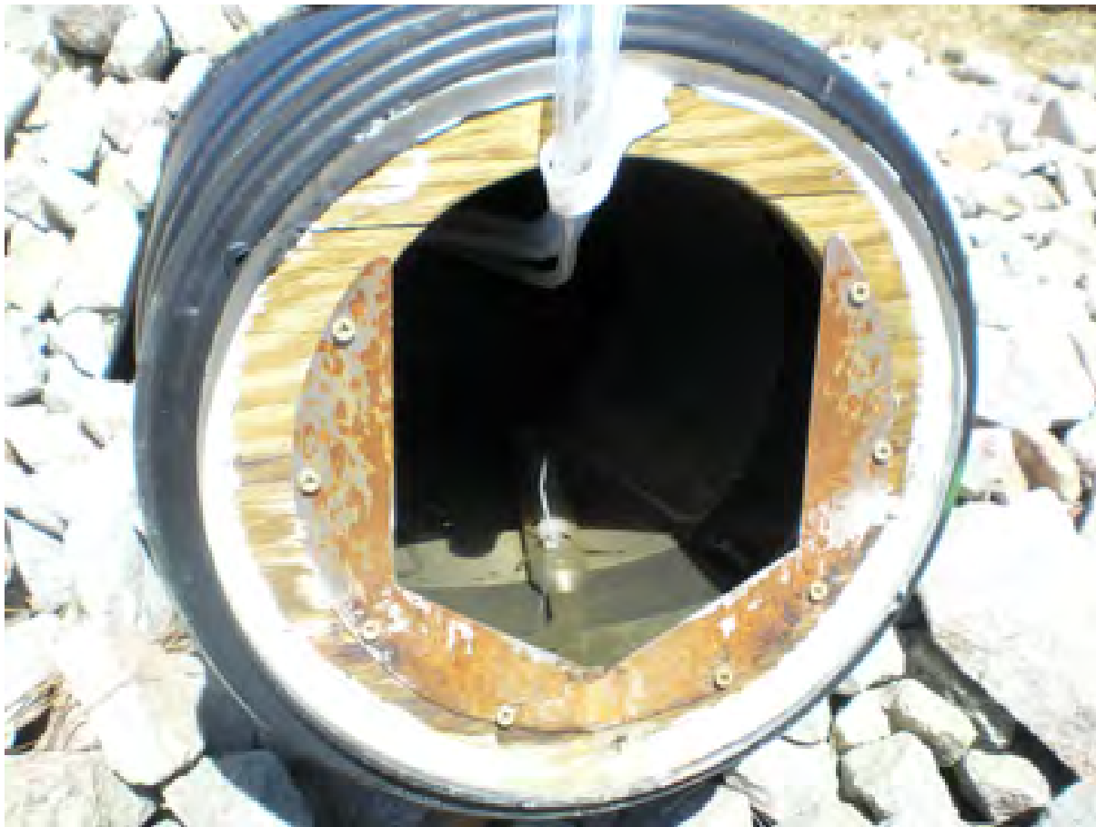
Figure 4-12. Inflow pipe to a bioretention area equipped with compound weir and bubbler for flow measurement. Water quality sampling tube and strainer are visible inside pipe.
