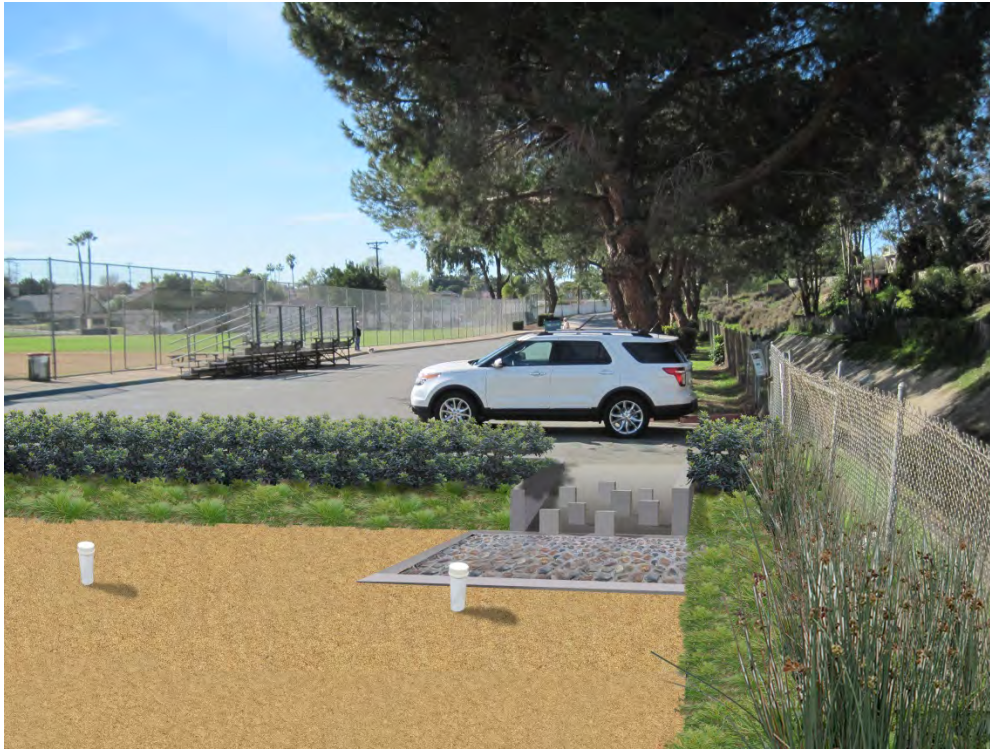
Figure 3-36. Surface sand filter with concrete energy dissipater (rendering).
