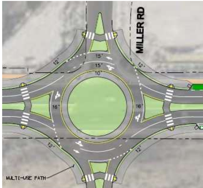
Image 2: Conceptual design of two-lane roundabout at Miller Road
