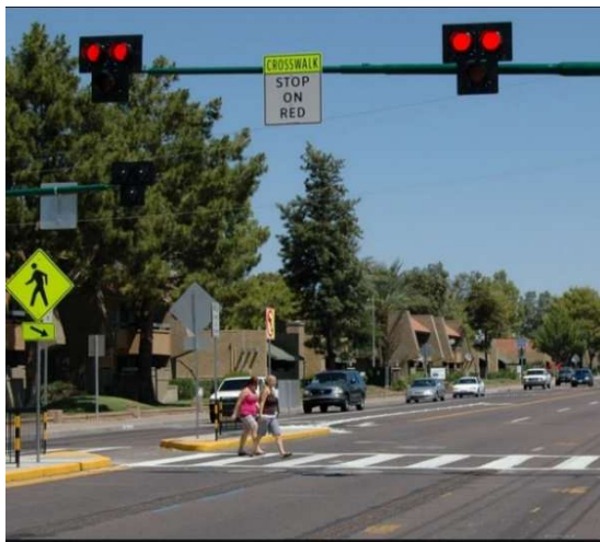
Photo 6: Example of HAWK signal at controlled crosswalk (left) and signal-controlled crosswalk (right)
