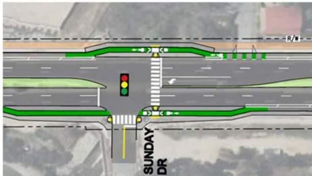
Image 3: Conceptual design of traffic signal with curb extension
