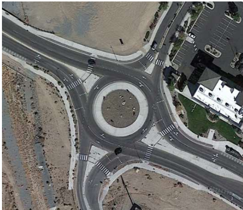
Photo 4: Typical two-lane roundabout with splitter islands (Sparks, Nevada)
