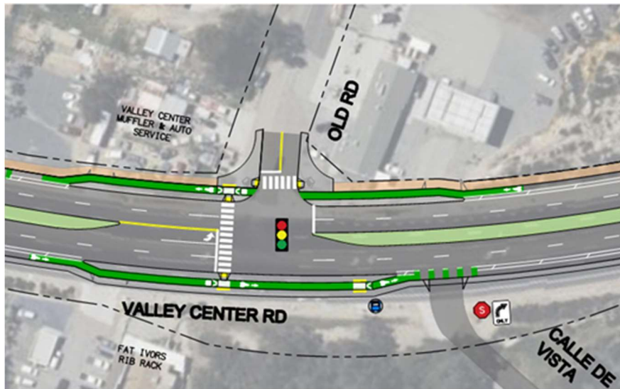
Image 1: Conceptual design of traffic signal at Old Road
