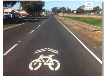
Sharrow and "Bike May Use Full Lane" Sign on Coastal Highway 101 in Encinitas
