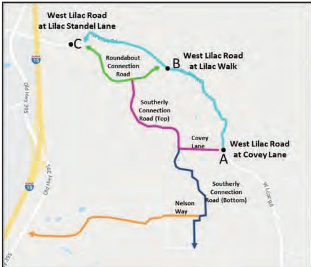
Figure 1. Existing and Proposed Parallel Road Network. Note the light blue existing road network and its proximity to the steeper slopes to the north. The proposed alternative road system (magenta, green, dark blue and orange) parallels West Lilac Road to the north, but is set back considerably and located within hardened (less burnable) landscapes. The routes provide additional flexibility and optionality to the west and south that do not currently exist.
