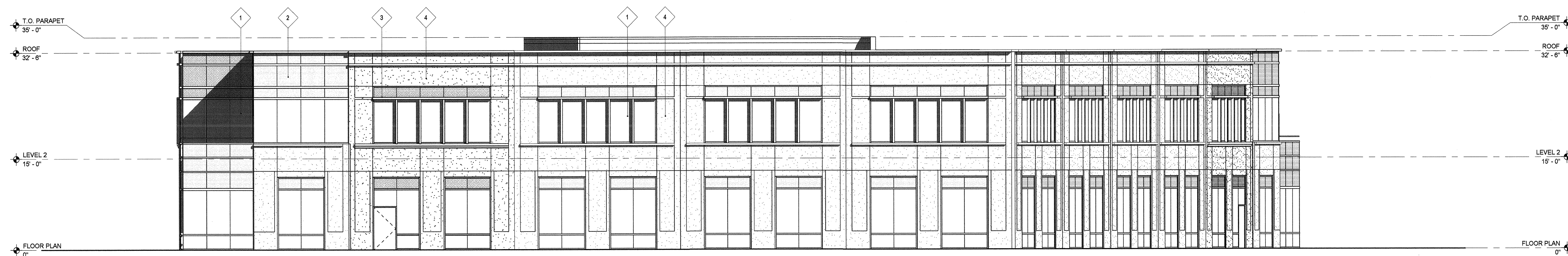
3 BUILDING A - WEST ELEVATION 1/8" = 1'-0"
