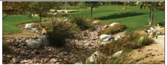
Storm Water Management and Low Water Use Landscapes - Run-off shall be managed through state-of-the-art infiltration design techniques and native and Mediterranean planting shall be used in common areas to reduce irrigation needs.
