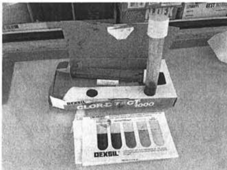
Field Test Results- show the oil does not contain chlorinated solvents
