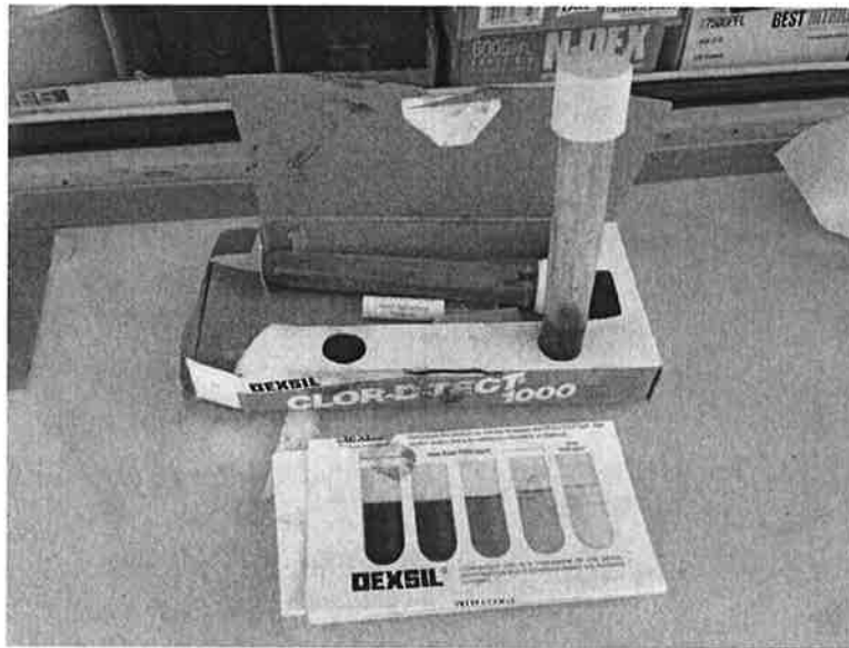
Field Test Results- show the oil does not contain chlorinated solvents
