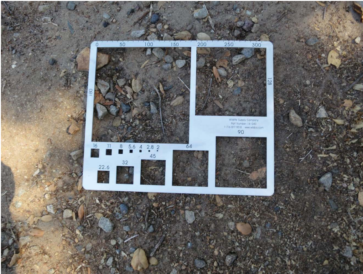
Figure 27. Gravelometer within Reach 3
