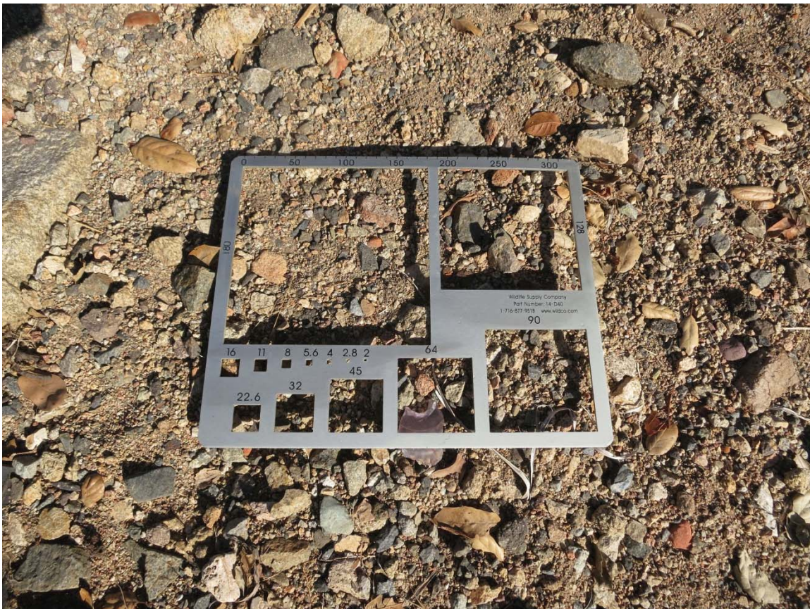
Figure 26. Gravelometer within Reach 2
