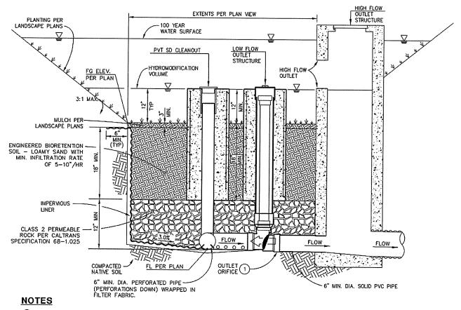
6" PVC RECTORSEAL CLEAN CHECK EXTENDABLE BACKWATER VALVE, OR EQUIVALENT (HYDROMODIFICATION OUTLET CONTROL STRUCTURE), WITH LOW FLOW ORIFICE.
