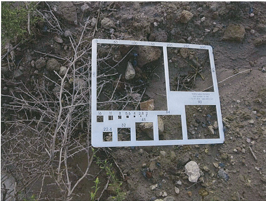
Figure 13. Gravelometer on Channel Bed Near Upstream End of Study Area
