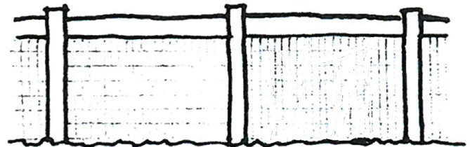
POST AND MESH FENCE
