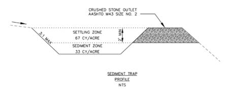
The sediment storage volume for a sediment basin should be calculated using the RUSLE equation to determine the annual sediment loading appropriate for a basin designed to be maintained once per year. The sediment storage zone should be at least 1 ft deep. The settling storage volume for a sediment basin should be calculated from a 2-year storm event with a settling zone at least 2 ft deep.
