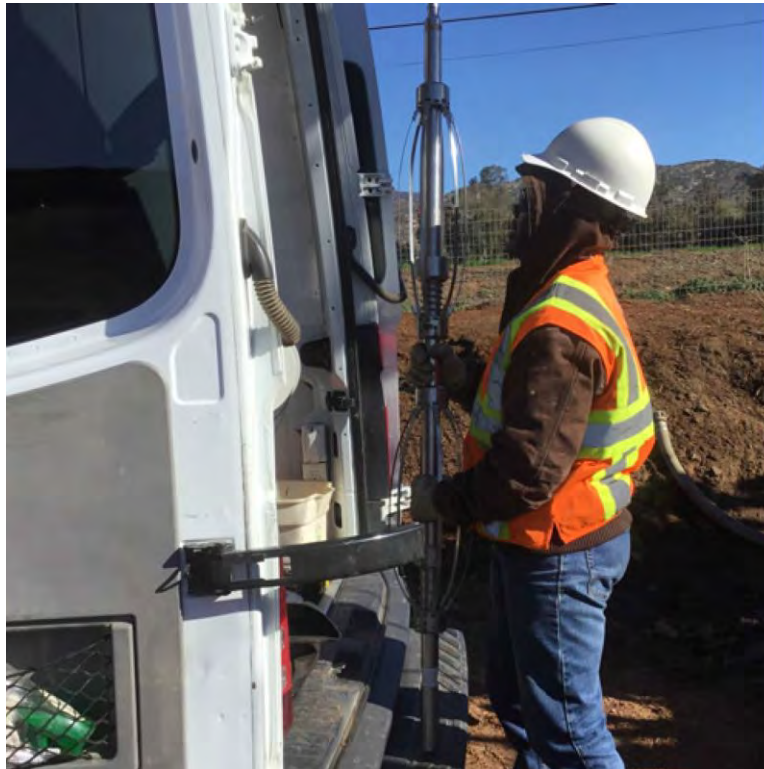
Photograph 7 - Optical televiewer equipment used for geophysical borehole logging.
