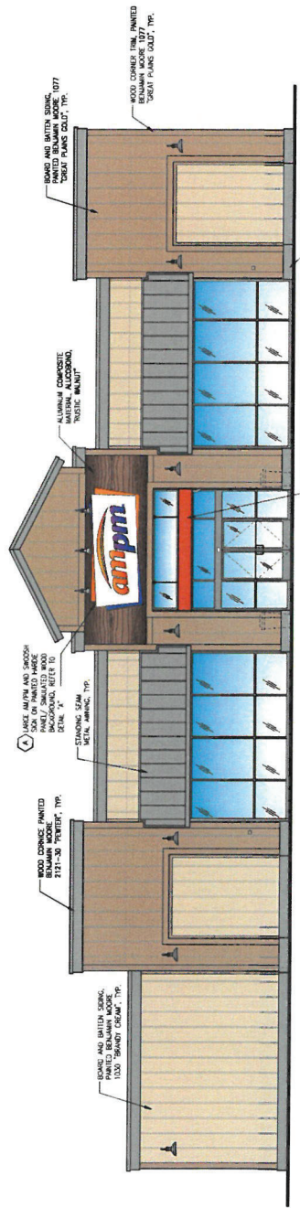
1 PROPOSED NORTH ELEVATION - FACING VALLEY CENTER ROAD SCALE: 3/16"=1'-0"
