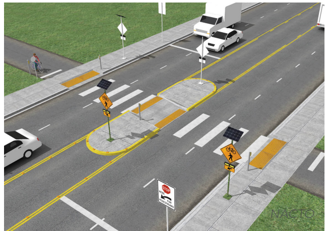
Examples of a Rectangular Rapid Flashing Beacons (RRFB)
