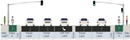
\*A sidewalk is proposed within the area of the curb extension and the Heritage Irail would remain, outside of the curb extension area.
