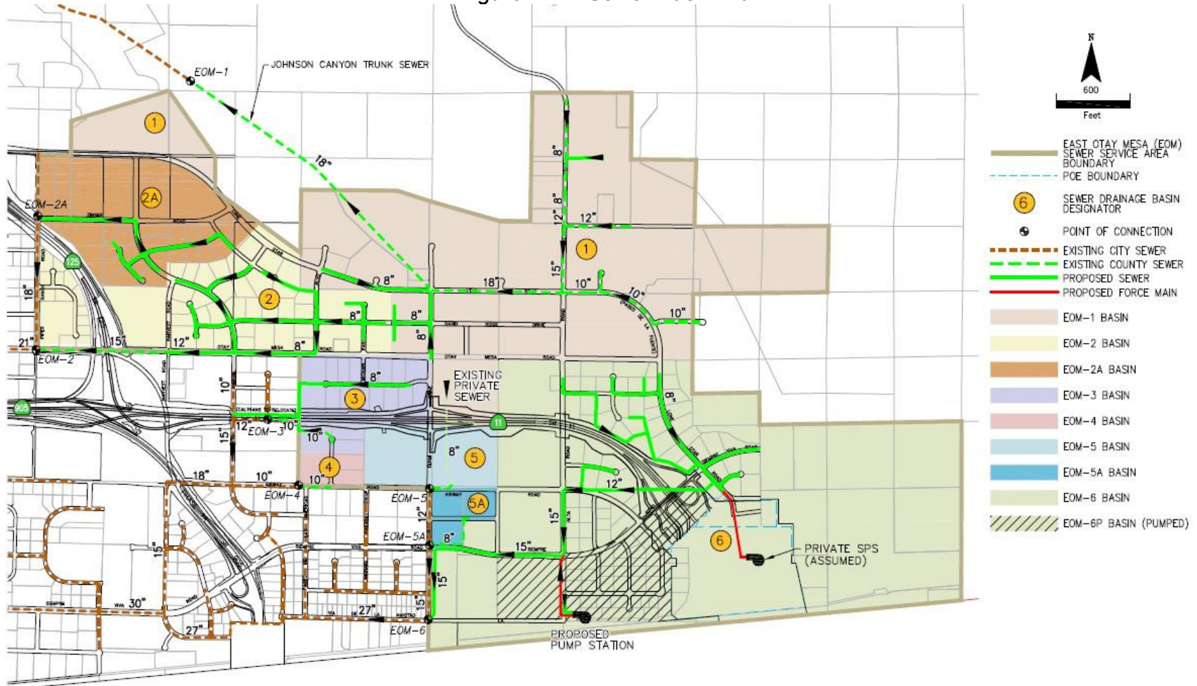
Figure 2.4-1 Sewer Basin Plan
