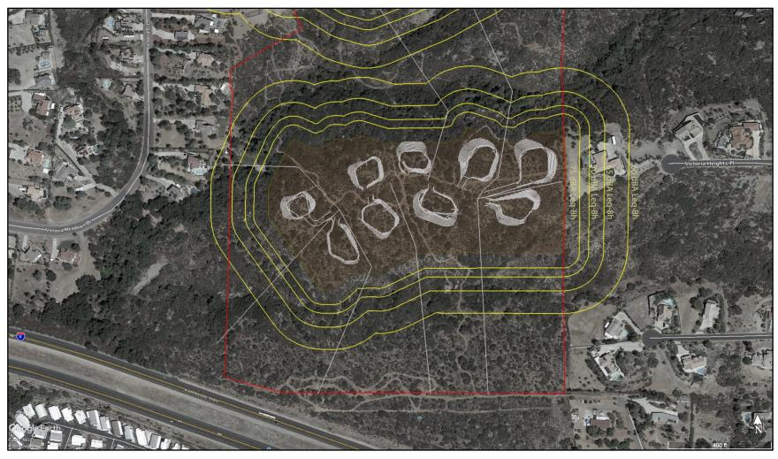
FIGURE 8b: Expected Southerly Construction Noise Exposure Map (ISE 1/19)
