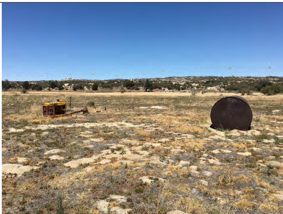
Photo 20. One of the wells with a pump and AST on the former ranchland. Well was no longer functional and appeared filled in.
