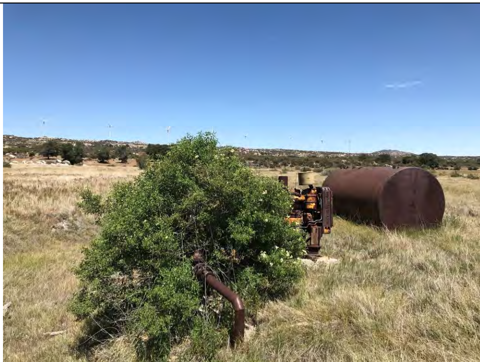
Photo 23. Larger motor and AST with second well south of the smaller well. Well was covered by a bush. Label on AST was rusted over but appeared to be roughly 3-4,000 gallon capacity.
