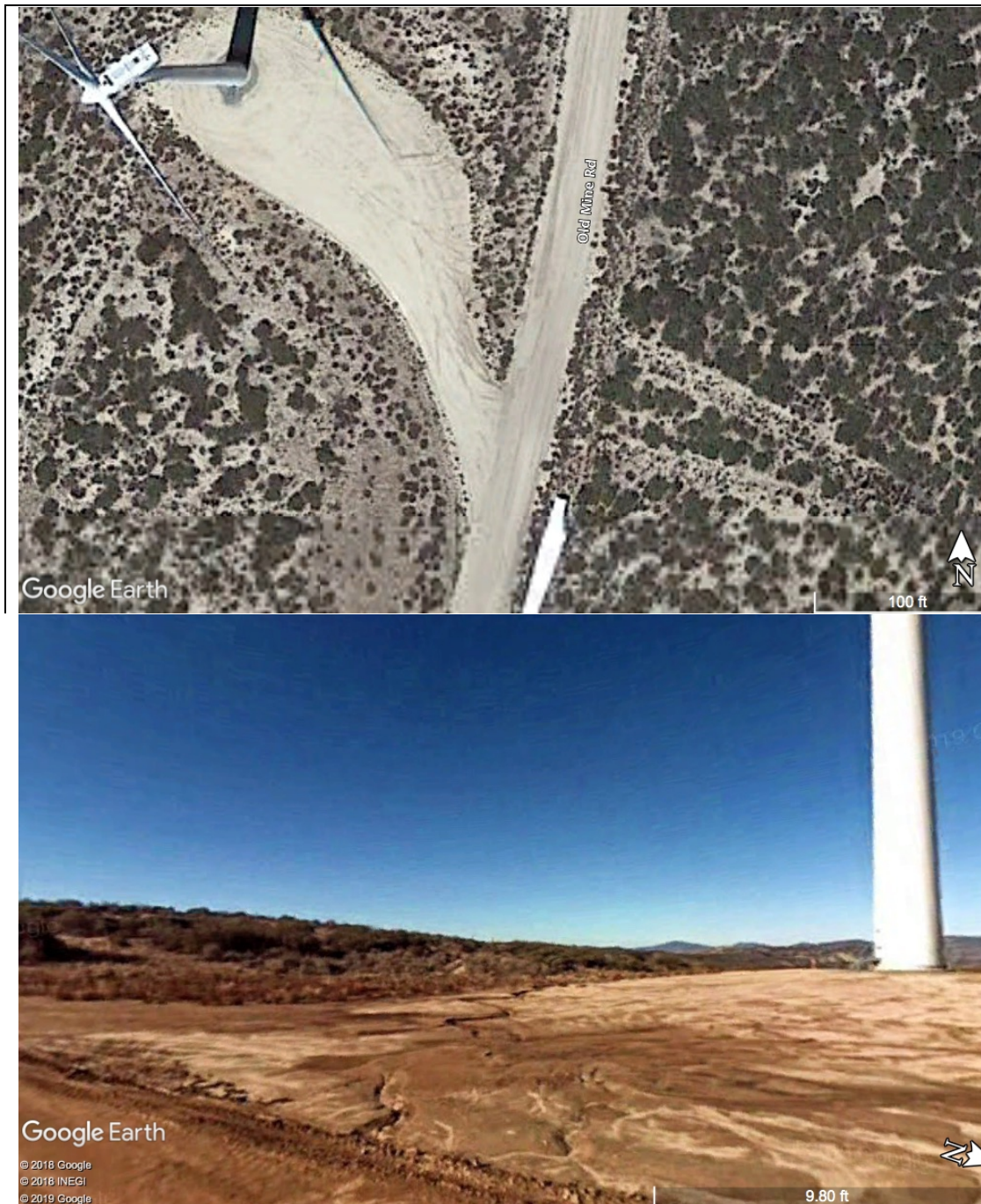
Figure 4. Erosion at Kumeyaay Wind Farm turbine pad from above (top image) and street view (bottom image).
