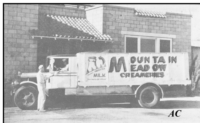
Mountain Meadow creamery has added this General Motors truck equipped with an 1100-gallon stainless steel lined, cork insulated thermos tank to its fleet, for carrying milk from its Jacumba ranch to San Diego in three hours. Milk is maintained at even temperature and is unloaded by forced air pressure. The firm also has added Divo enclosed type milk delivery trucks.
