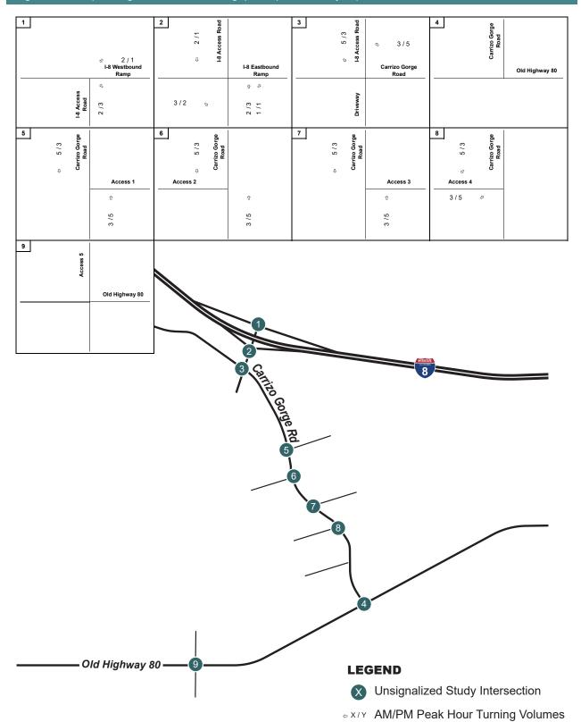
Figure 5-3 Existing (2019) Plus Construction Traffic Peak Hour Volumes
