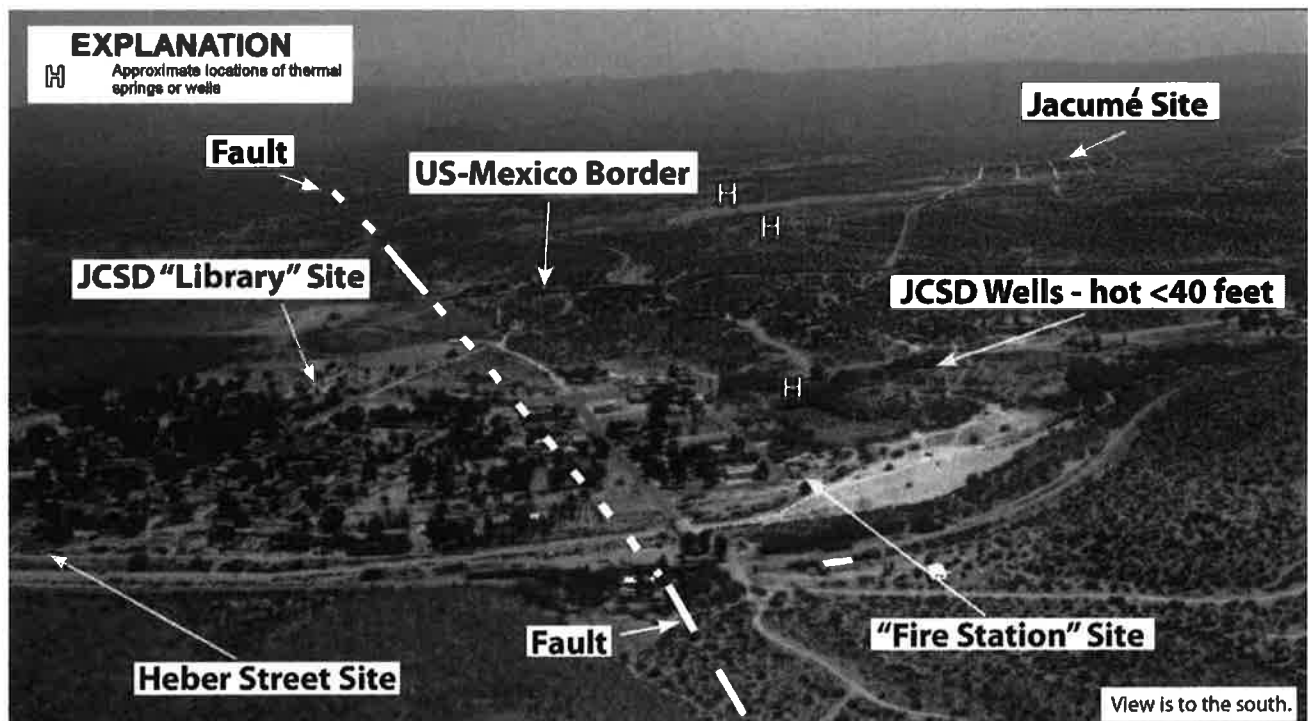
Figure 8. Oblique aerial photograph of the Jacumba area showing thermal springs and wells
