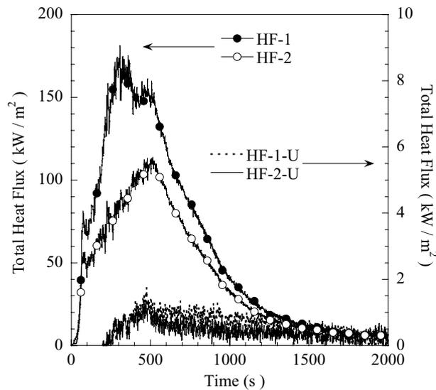
**Figure 5. Temporal evolution of the total heat flux measurements, both at the exposed and unexposed face.**
