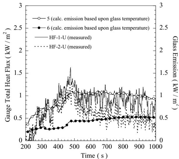
**Figure 6. Temporal evolution of the calculated emission based upon glass temperature. The temporal evolution of the measured total heat flux at the unexposed glass surface is shown as well.**
