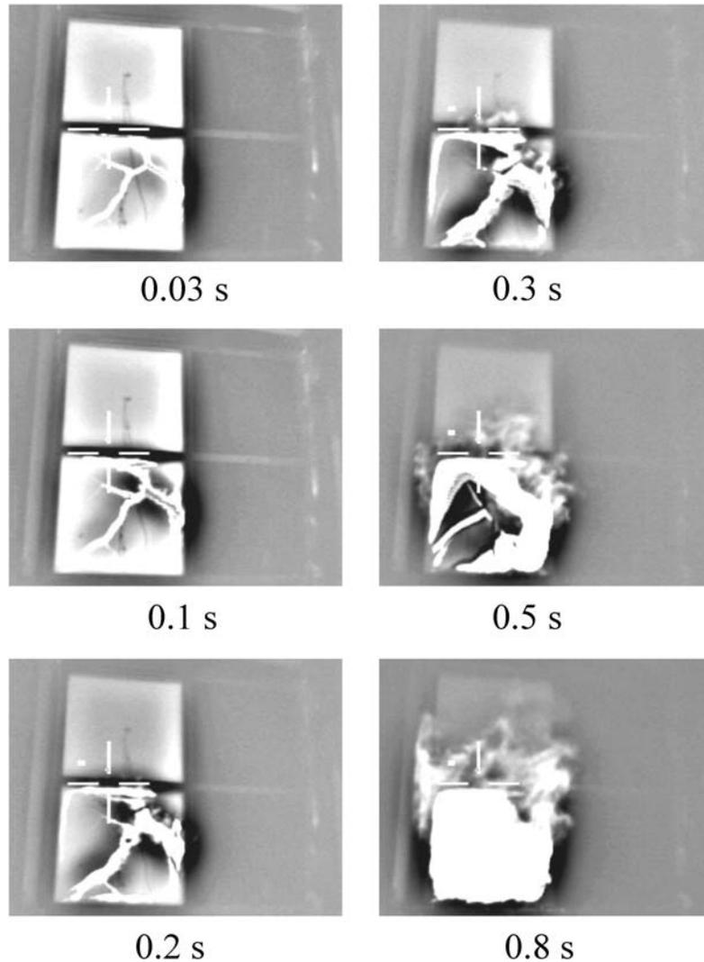
**Figure 3. (a) Temporal evolution of the glass fall out as seen with the infra-red camera. The camera is focused on the unexposed face.**
