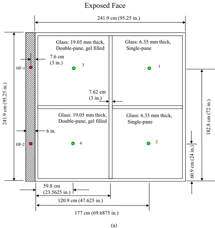
**Figure 1. (a) Drawing of glass wall assembly showing the exposed face.(b) Drawing of the glass wall assembly showing the unexposed face.(c) Schematic of compartment used for the fire test. (Continued in next page.)**
