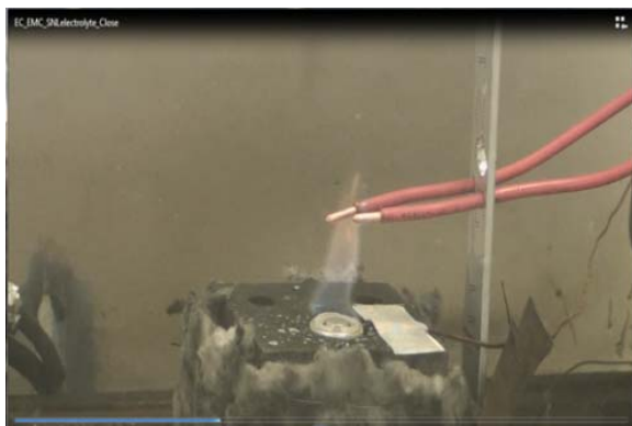
Figure 11. EC:EMC (3:7 w%)-1.2M LiPF 6 is mildly flammable.
