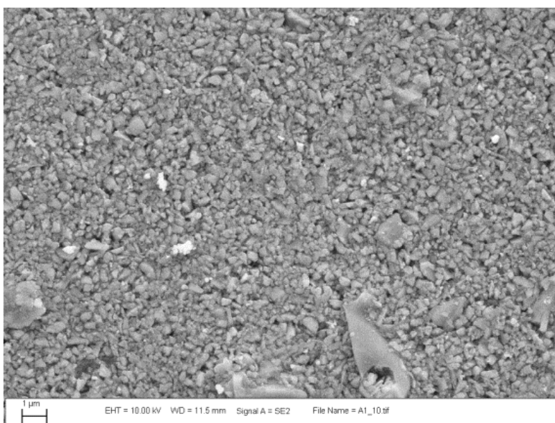
Figure 39. 10% binder on tabular alumina, low porosity. Scale bar represents 1 μm.
