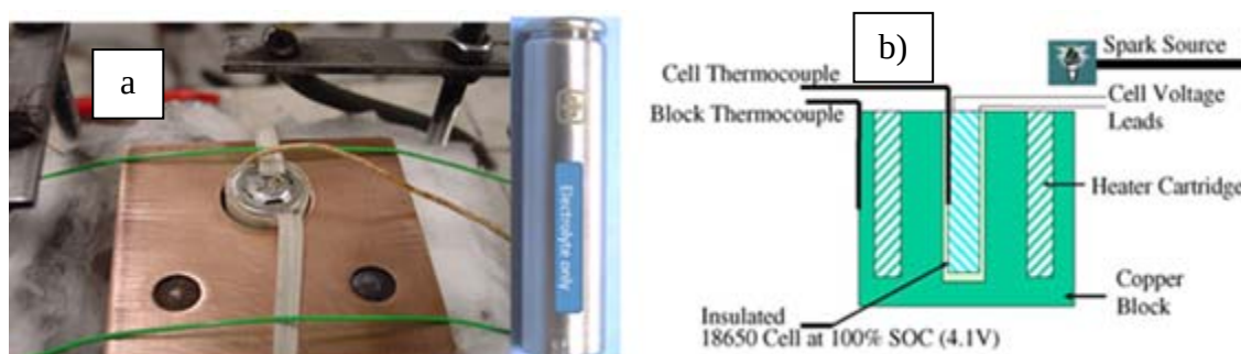
Figure 10. Experimental setup showing: a) picture of the copper heater block used and b) line drawing of the experimental setup.
