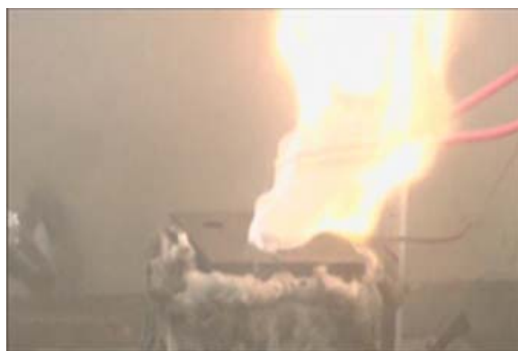
Figure 12. EC:DEC (5:95 V%)-1M LiPF 6 is violently flammable.
