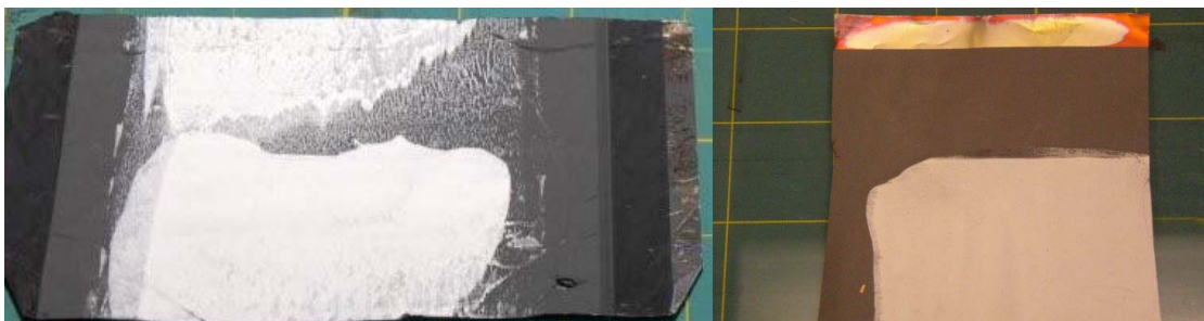
Figure 40. Ceramic separator cast directly onto cell electrodes.
