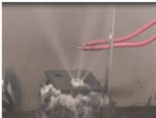
Figure 13. EC:DEC:TMMP (5:45:50 v%)-1M LiBETI is nonflammable.
