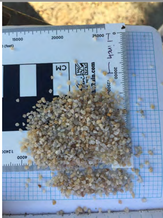
Photograph 8. Sample of Cal-Silica 8 x 16 silica sand filter pack
