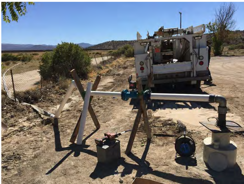
Photograph 18. Highland Center well pump-testing.
