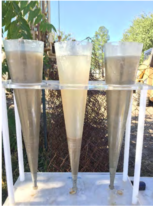
Photograph 15. Initial Imhoff cone samples from well development.
