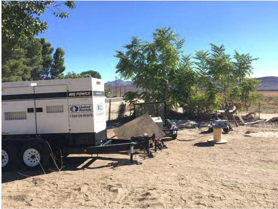
Photograph 19. Equipment setup for well pump-testing.
