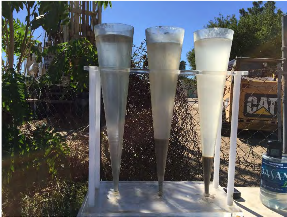
Photograph 17. Well development, Imhoff cone samples.
