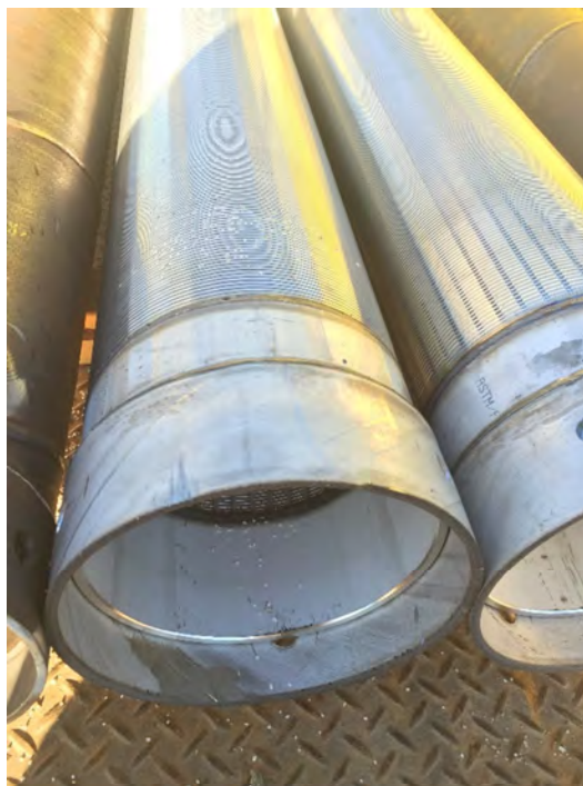
Photograph 6. Johnson 0.05-inch slot, 8 5/8-inch diameter stainless steel wire-wrap screen.
