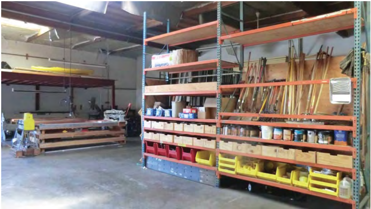
Interior of Shadowcrest Roofing operations area; supplies and hand-tools used in roof-related contracting. At rear are brakes for forming sheet metal flashings, etc.
