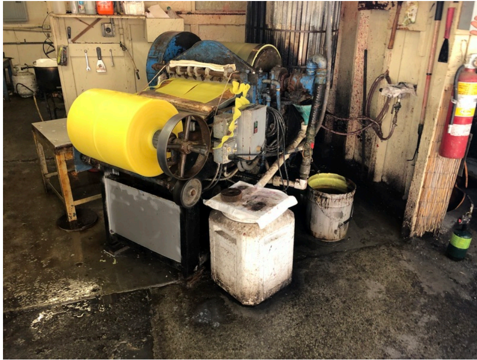
29. Honeycomb candle making machine
