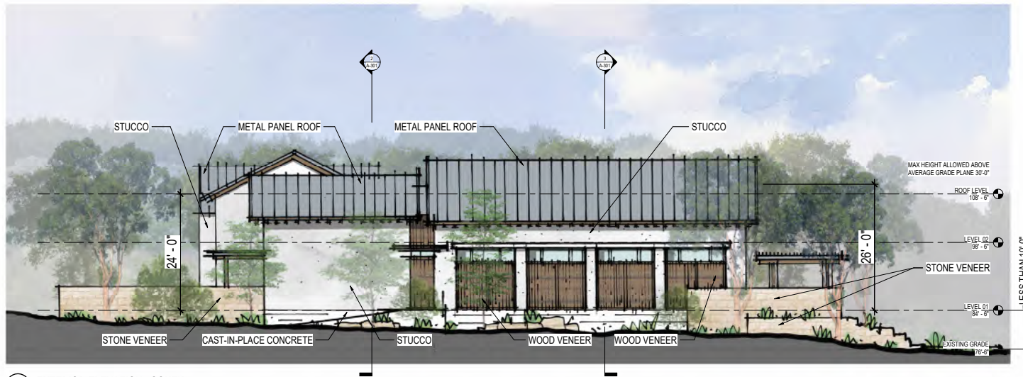
1 EXTERIOR ELEVATION - SOUTH SCALE: 1/8" = 1'-0"
