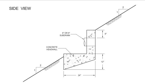
NOTE: HEADWALL SHOULD OUTLET AT TOE OF FILL SLOPE OR INTO CONTROLLED SURFACE DRAINAGE
