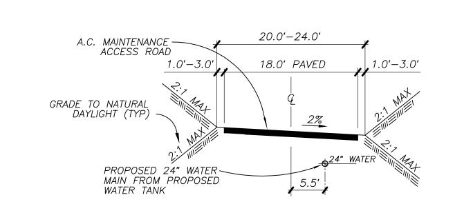
MAINTENANCE ACCESS ROAD TO PROPOSED WATER TANK 1.5:1 GRADIENT SLOPES ALLOWED IN "CUT" SLOPES
