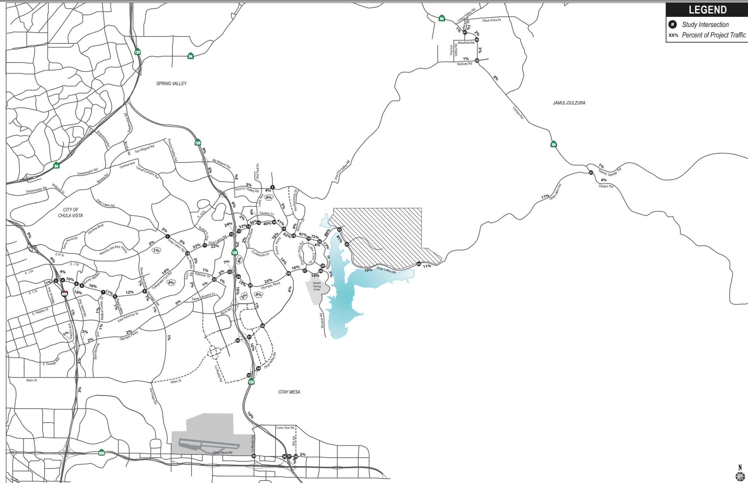
Figure 2.9-3 Project Trip Distribution - Buildout Cumulative (Year 2025) Network
