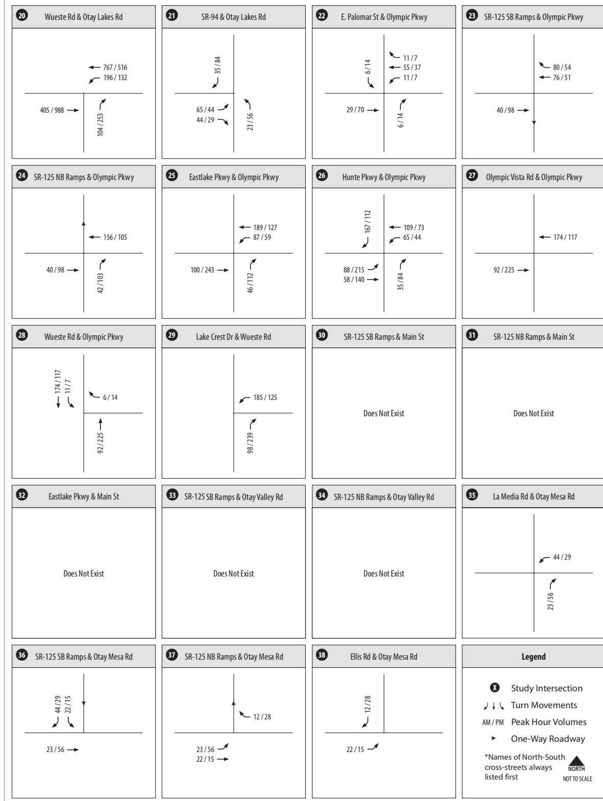
Figure 2.9-10 Project (Buildout) Trip Assignment (Intersection) - Cumulative (Year 2025) Network (Intersections 20-38)
